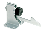
202F-B Adjustable gate stop. Slot to accommodate up to a 2-1/2" gate frame. mounted via screws. 5-1/8" high.
