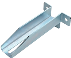
354-330 Adjustable wall support. 13" long. Recommended spacing 27-1/2" apart. Galvanized
