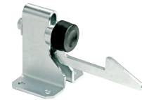
202F-B Adjustable gate stop. Slot to accommodate up to a 2-1/2" gate frame, mounted via screws. 5-1/8" high.
